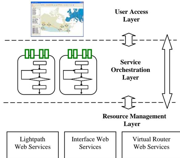
Figure 1 UCLP system architecture in three layers
